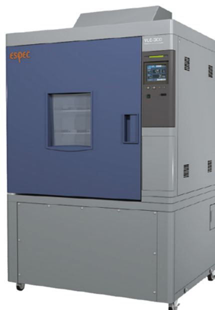
Airborne Test Chamber for Batteries
